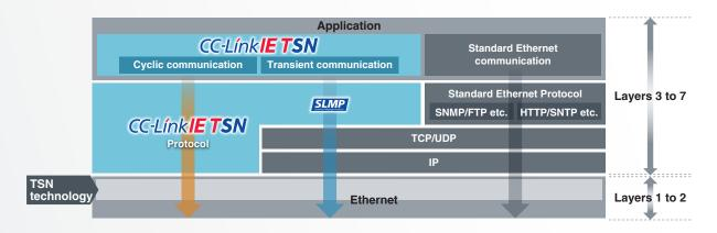
TSN consists of multiple international standards. The major standards are IEEE802.1AS (which defines the time synchronization method) and IEEE802.1Qbv (which defines the time sharing method). Combining these to the Ethernet standard enables punctuality, ensuring transmission within a given period of time, and mixed implementation with other communication protocols.
